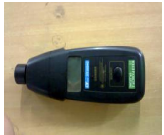
Tachometer for measuring engine RPM
